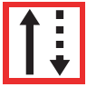
Must maintain a course on the port side of the navigation channel
